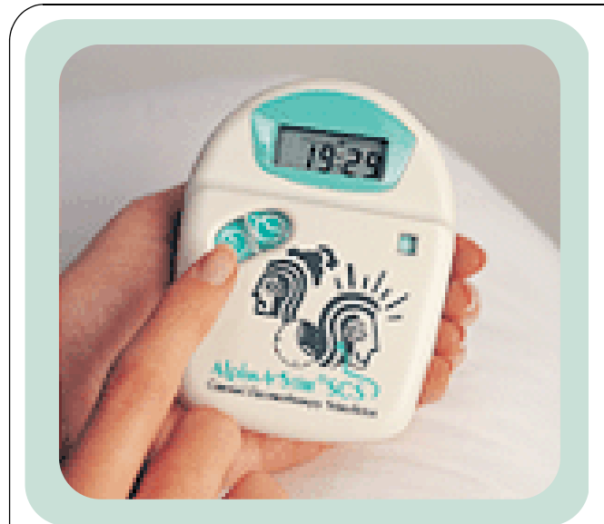
Figure 2. Alpha-Stim® Stress Control System microcurrent stimulator. Reproduced with permission from Electromedical Products International, Inc. (TX, USA); www.alpha-stim.com.
